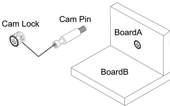
To assemble this product hardware called Cam Lock Fasteners are used. The below is information on how these work. Cam Locks are fasteners used to join two boards together, usually the edge of one board (A) to the flat side of another board (B).
