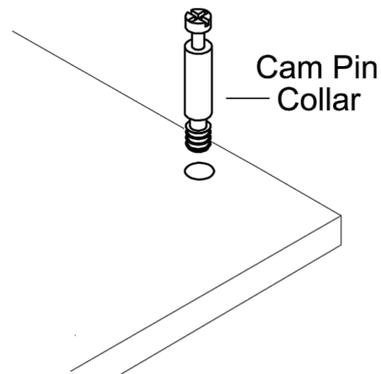
The Cam Pin is inserted into the flat side of a board, it is important that: The cam pin is kept vertical and is not put in on an angle. Cam pin is to be inserted up to collar (Do Not Overtighten) Too far and it wont catch the Cam Lock (Do Not Overtighten) Not enough and the resulting product will not be stable.
