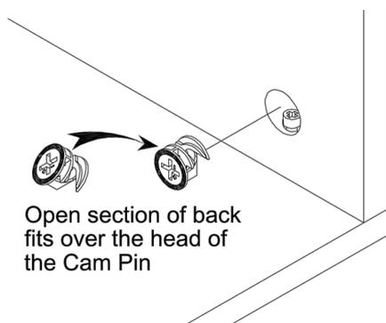
Insert the Cam Lock into the large hole so the opening of the "C" fits over the head of the Cam Pin. You must ensure that the Cam Lock is pushed to the bottom of the hole to catch the top of the Cam Pin.
